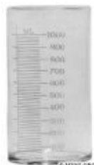
No. 745 - 1000 CC Childow Expansion Jar Graduated in 20cc Divisions (Crystal)
